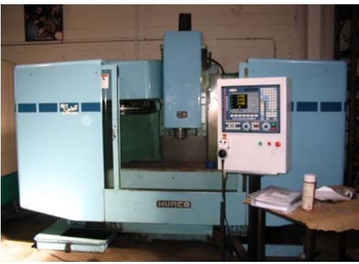
CNC Control Retrofit
